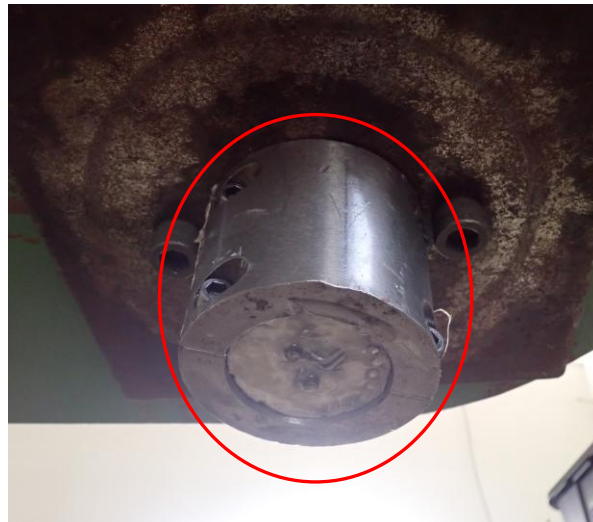
Figure 3-2: Photograph showing the epoxy filled socket fixture (ellipse) utilized to terminate the conductor at both ends.
