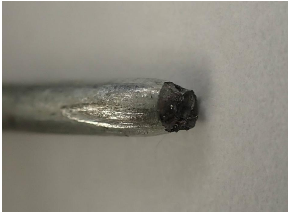
Figure 2-10: Close-up view of a representative example of the fracture failure morphology observed for the steel reinforcing core strands associated with conductor EL-1. The morphology was characterized by a tapered (necked) interval immediately adjacent to the strand fracture surface.
