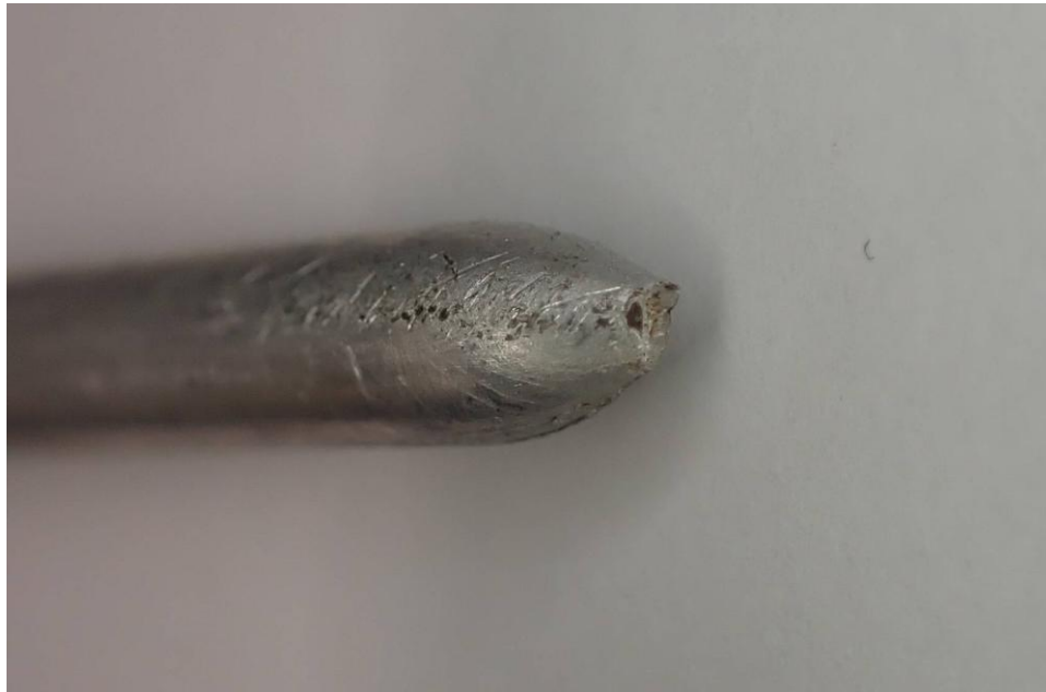
Figure 2-6: Close-up view of a representative example of the first fracture failure morphology observed for the aluminum strands associated with conductor EL-1. The first morphology was characterized by a tapered (necked) interval immediately adjacent to the strand fracture surface.
