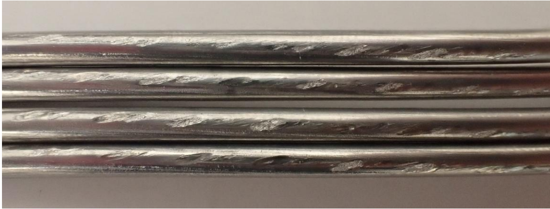
Figure 3-10: Close-up view of a representative example of the strand on strand brinelling (localized deformation) observed on the individual aluminum wire strands subsequent to uniaxial tension testing.
