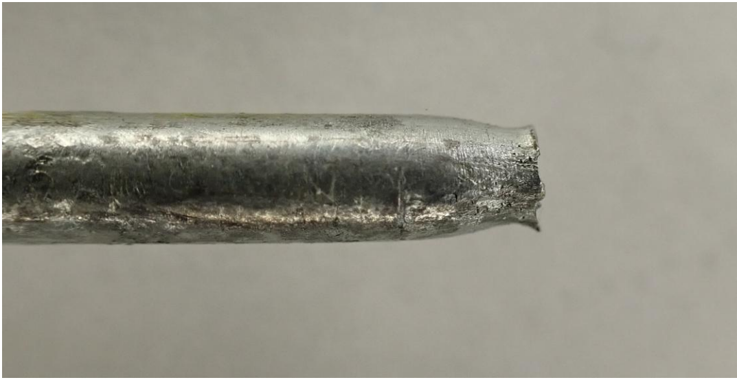
Figure 3-8: Close-up view of a representative example of the fracture failure morphology observed for the steel reinforcing core strands subsequent to uniaxial tension testing. The morphology was characterized by a tapered (necked) interval immediately adjacent to the strand fracture surface.
