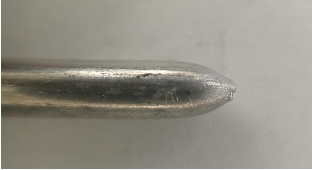
Figure 3-6: Close-up view of a representative example of the first fracture failure morphology observed for the aluminum strands subsequent to uniaxial tension testing. The first morphology was characterized by a tapered (necked) interval immediately adjacent to the strand fracture surface.
