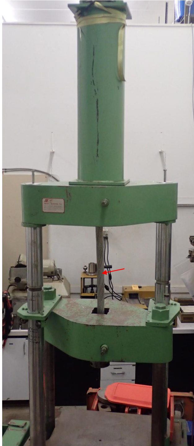
Figure 3-3: Photograph showing the load train utilized to test the intact service exposed conductor in uniaxial tension (the arrow indicates the conductor).
