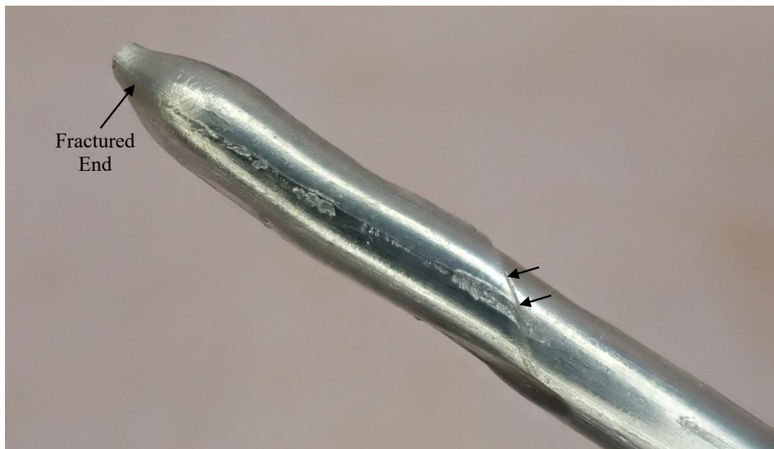
Figure 2-8: Close-up view of a representative example of a partial through wire indication detected in an aluminum strand (arrows).
